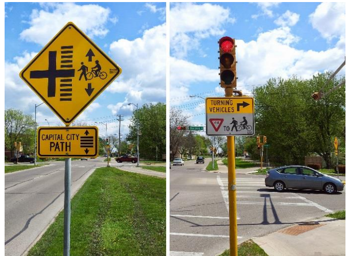
Sidepaths can present conflicts between people bicycling and people driving, especially at intersections and driveway crossings (above). Steps can be taken to mitigate these conflicts. Examples include high-visibility pavement markings, specialized warning signs, and enhanced traffic signals (below).
